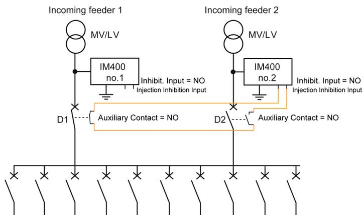
Using circuit breakers with normally closed (NC) auxiliary contacts:
