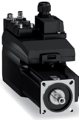
The **Lexium 32i** is an integrated servo drive and comprises motor, positioning controller, power electronics, fieldbus and “Safe Torque Off” safety function in an extremely compact single device.
