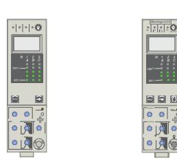
MicroLogic 7.0: selective + earth-leakage protection
