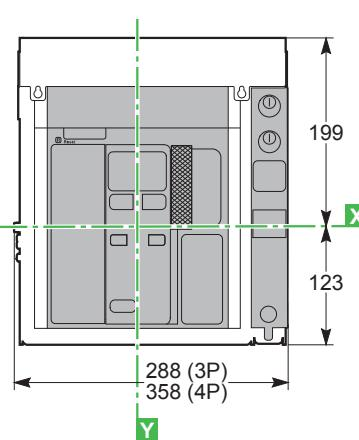
[1] the size of MasterPact MTZ1 is 13 mm, including spring charging handle deeper than MasterPact NT due to the bigger size of the new front cover. For MasterPact MTZ2/3 the difference is only 3 mm.
