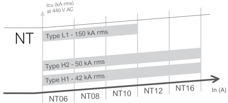
> MicroLogic A/E [1] Control Units for MasterPact NT
