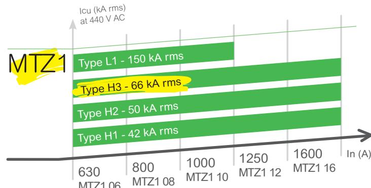
> MicroLogic X [3][4] Control Units for MasterPact MTZ1 Protection for ...
