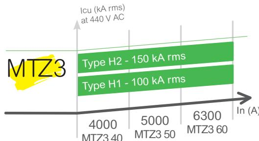
> MicroLogic X [3][4] Control Units for MasterPact MTZ3 Protection for ...
