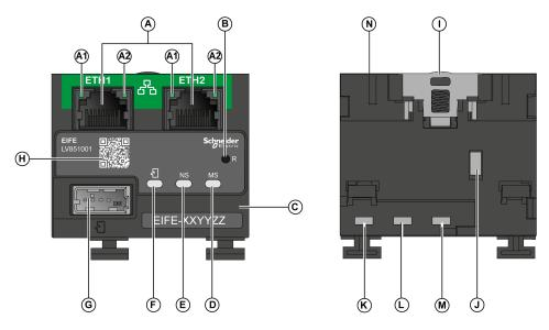
A Two RJ45 Ethernet ports
