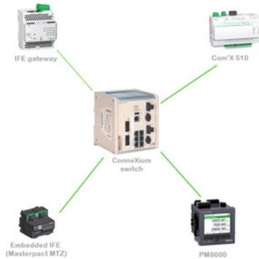
Star topology is a communication architecture in which each device is connected individually to a central node, generally a switch.
