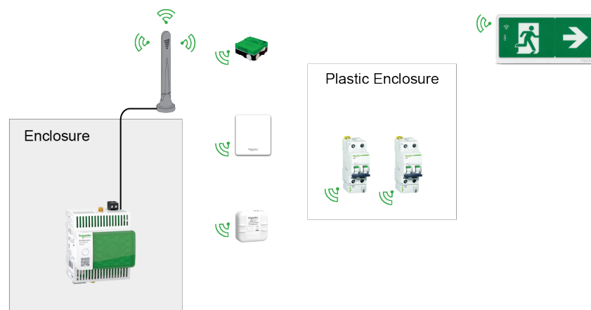
Illustration 8: Panel Server Advanced in an enclosure and wireless devices in an open field
