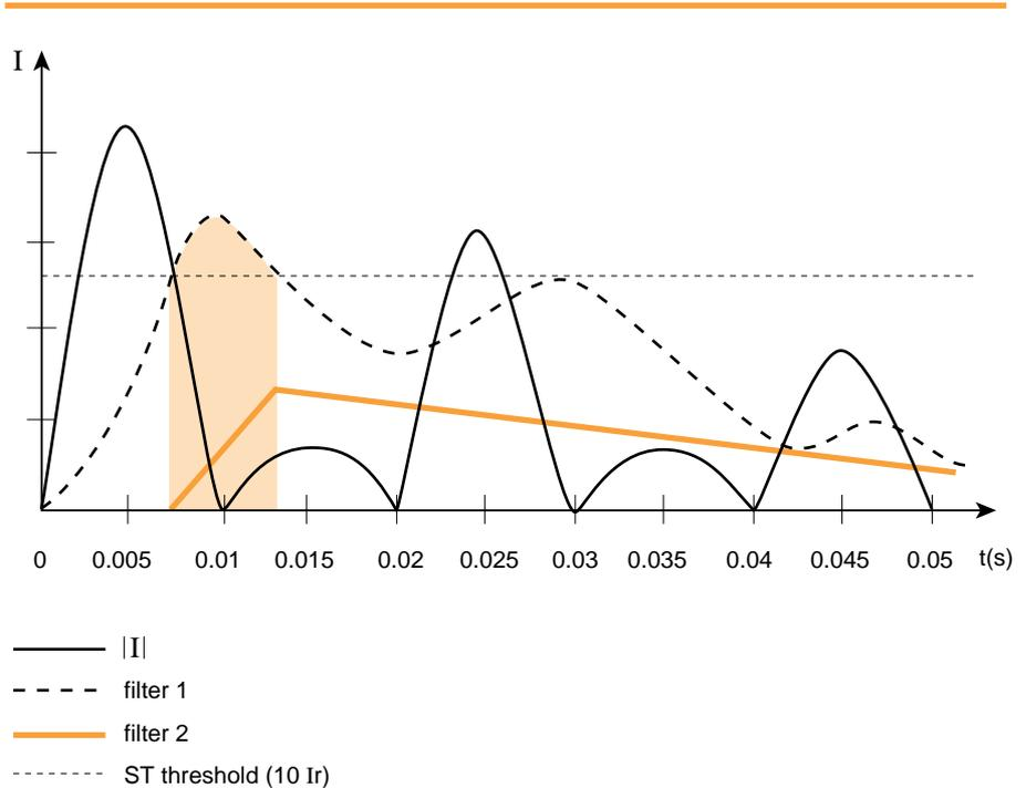
fig 15: transient current solved by «smoothing» the IIR filter.
