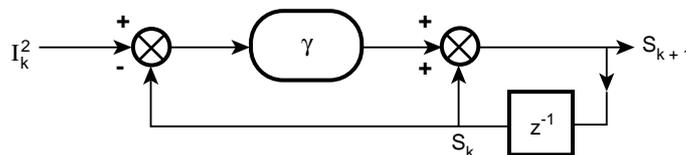
fig. 6: filtering algorithm (R) of the low pass digital filter.
