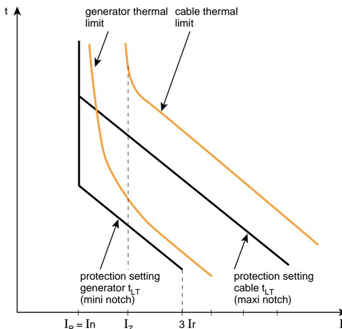
fig. 19: long time tripping curves of an electronic circuit-breaker protecting a cable or generator.
