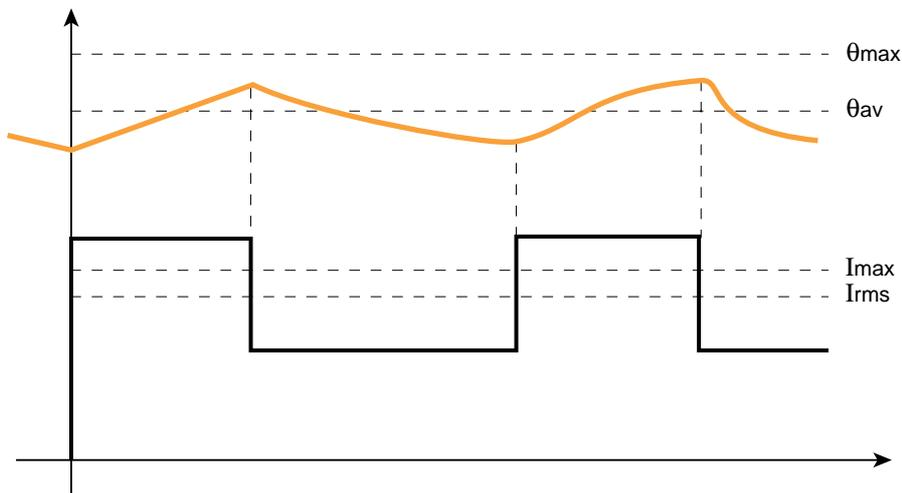
fig. 17: cyclic heating of a conductor with continuous load plus cyclic load.
