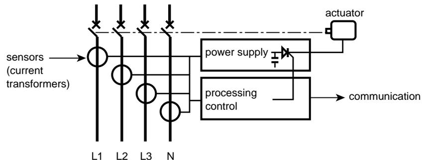
fig. 2: functional modules of a control unit.
