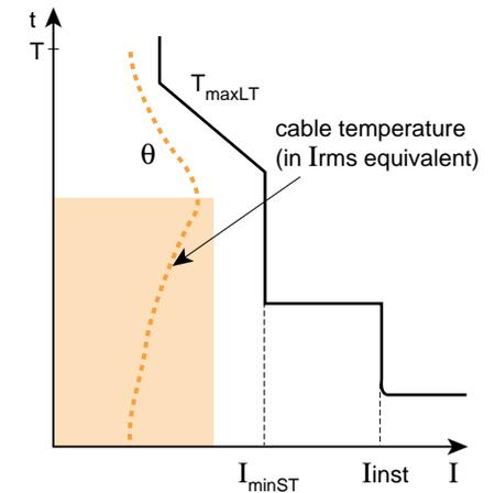
fig. 18: Long and Short Time settings for strong, short or meak, long cyclic loads (steady state).
