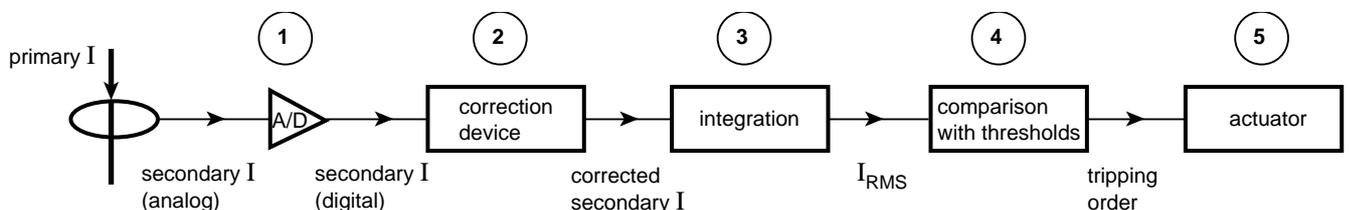
fig. 3: functional diagram.
