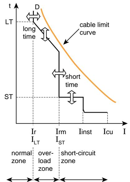
fig. 9: electronic circuit-breaker tripping curves.
