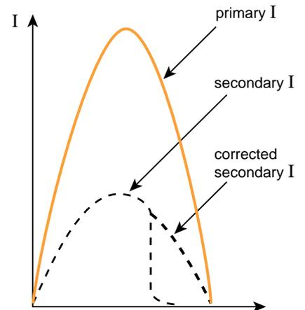
fig. 4: sampling and correction of CT saturation (if any).
