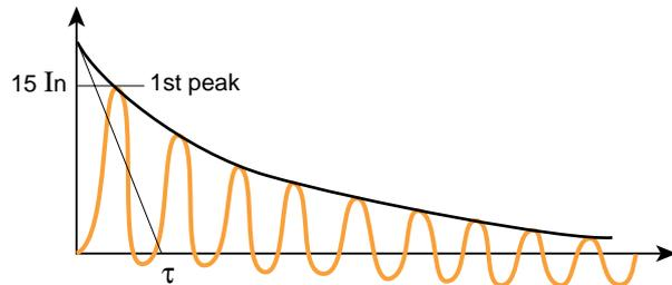
fig 13: transformer energising.
