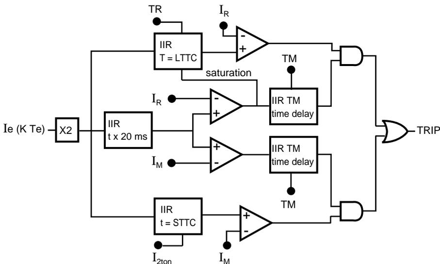
fig. 8: structure of the long and short delay filter assembly.
