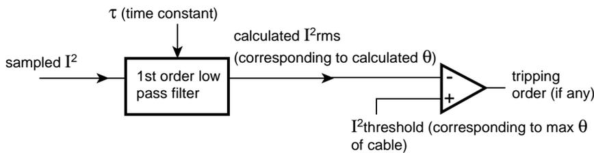
fig. 7: making the Long Time (LT) function.
