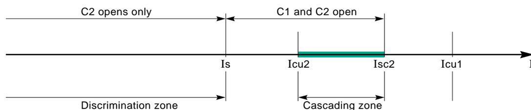
**fig. 7:** The principle of cascading between 2 circuit breakers, breaker C2 whose breaking capacity  $I_{cu2}$  is less than the three-phase short-circuit current at its terminals ( $I_{sc2}$ ), is protected or assisted by breaker C1.
