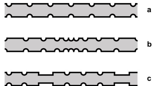
**Fig. 13:** different types of notching.
