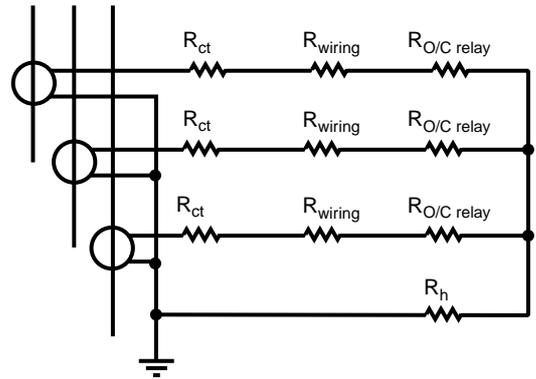
**Fig. 8** : internal and load impedances of a CT.
