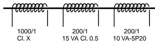
**Fig. 7** : example of poor understanding between the customer and the CT manufacturer.
