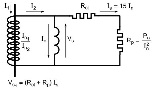
**Fig. 4** : calculating the characteristic voltage of a CT.
