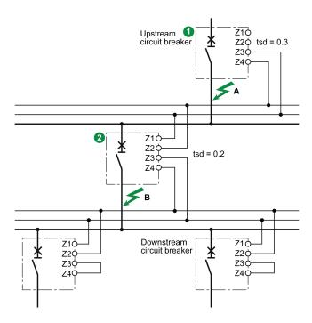
**NOTE:** On circuit breaker 1, the tsd and tg tripping delays must not be set to zero because this would make selectivity impossible.
